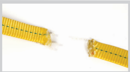
Traditional webbing lifeline (with energy absorber) failure
