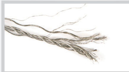
Traditional cable lifeline (with energy absorber) failure
