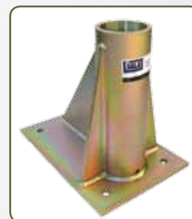
8530267 BOLT-ON FLOOR BASE Zinc plated steel construction. Bolts to steel and concrete horizontal surfaces.
