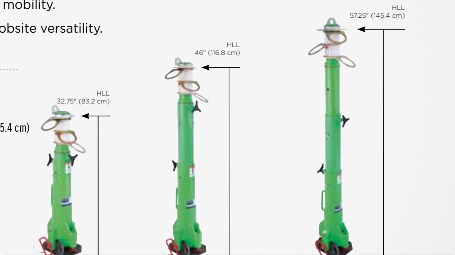
Telescoping design: Overall height can be adjusted from 32.75" (83.2 cm) to 57.25" (145.4 cm)
