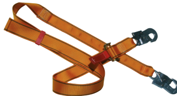
Web work positioning 45 mm lanyard, particularly suited to work on posts (wood or concrete). Easy to adjust roll bar buckle, even with one hand. Rigid section to facilitate passing the end of the strap around the pole.
